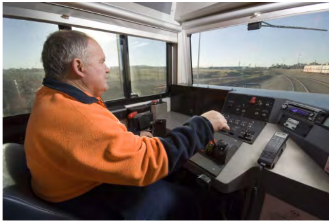
Driver in cab—right hand on power/deadman's handle
