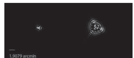
Figure 3. Higher-order aberration point spread functions (PSFs) from an eye with -3.00 D of spherical myopia at baseline (left) and one month after orthokeratology (right). Change in spherical aberration = 0.24 microns (5 mm pupil diameter). 55
