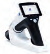
VISUSCOUT 100 Hand-held, rechargeable 5 megapixel fundus camera.
