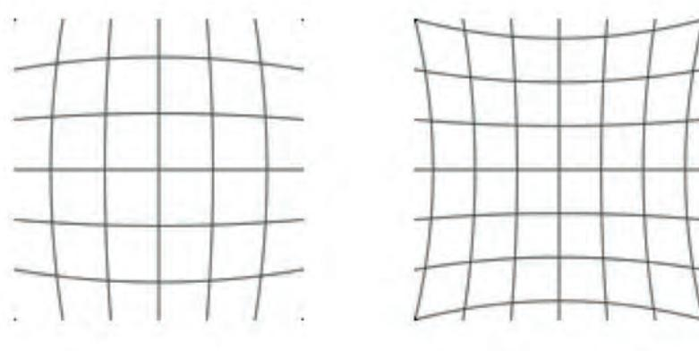
**Figure 2.** Barrel and pincushion distortion
