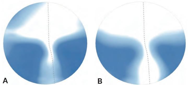
**Figure 3.** Restrictions in the vision zones of a traditional grind progressive lens caused by the base curve effect (as shown in Figure 3a).
