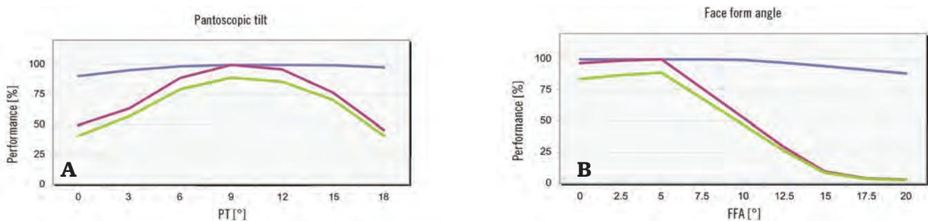
**Figure 4** The blue line represents a lens optimized for base curve effect and compensated for actual frame parameters. The purple line: a lens optimised for the base curve effect and standard frame parameters. The green line: a traditional grind lens.
