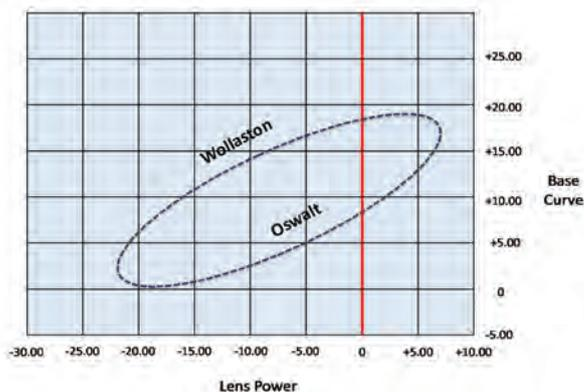
**Figure 1.** Tschernings ellipse for 1.5 index material
