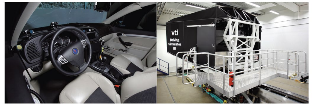
FIGURE 3. Picture of Sim III at VTI with the motion platform and the interior used in the test.
