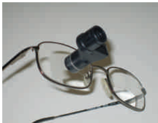
Figure 18. A and B: Lightweight Ocutech focusable Keplerian bioptic telescopes of 6x and 3x are available and suitable for longer duration wear. Their benefit is convenience for classroom use, theatre or ballet, gallery walking and sports. Smaller Galilean systems are less conspicuous in tinted carrier lenses but provide only half the comparable field width. Smartphone image zoom is often preferred for the quick view of direction signs or bus or tram numbers.
