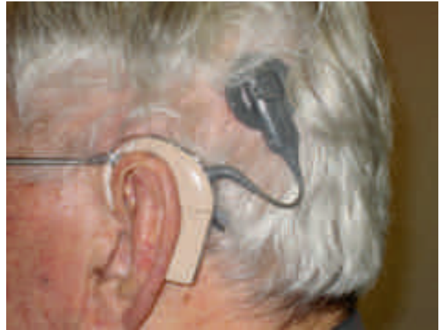
Figure 21. The bionic ear (cochlear implant) was developed in Melbourne and revolutionised the management of patients with profound deafness. The grey transducer above the ear attaches magnetically to an implanted transceiver under the skin. About 22 electrodes are implanted in the cochlea. The 'bionic team' of engineers and ophthalmologic surgeons is working on the bionic eye.
