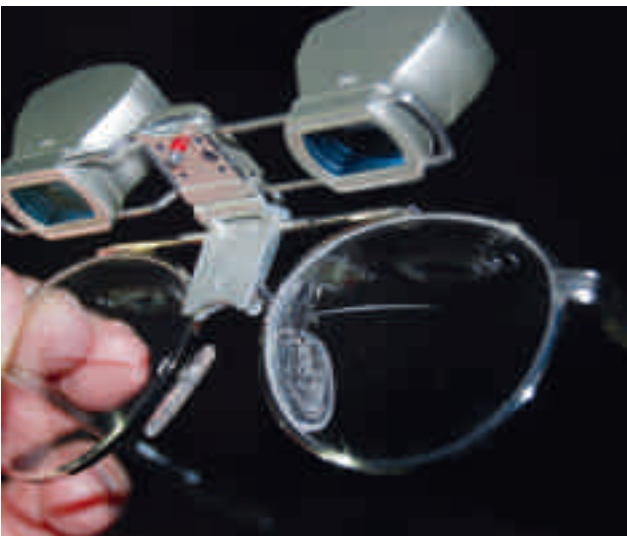
Figure 16. An alternative solution for near telescope use is to add power behind the telescope, about M^2 \times L . This telescope was made for a cellist who wished to see his music at 80 cm. The carrier lens had a +1.25 D near addition for this distance, while the upside-down bifocal segment behind the 2.2x bioptic telescope was an addition of 2.2^2 \times 1.25 \approx +6 D, less the +1.25 already in the lower section. A +4.5 D near add in the bifocal was our final solution. The conductor was slightly blurred.
