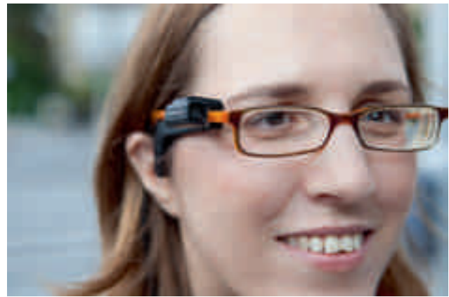
Figure 20. The OrCam is a portable camera and a pocket computer attached to the spectacle frame. It has text and face recognition, storing familiar objects (and people) for later recall.
